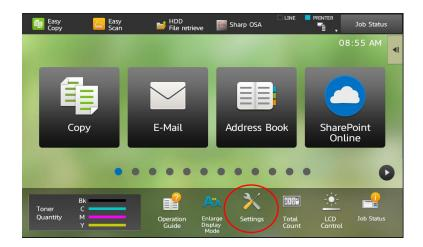
Select the **Settings** button on the device front panel.
